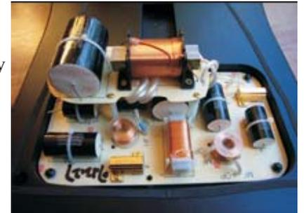
A passive crossover: coils, capacitors and resistors
